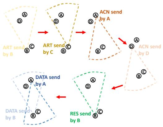
Fig. 4: Handshake procedure of VL-MAC
