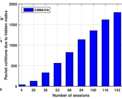
Fig. 7: Packets dropped due to hidden nodes
