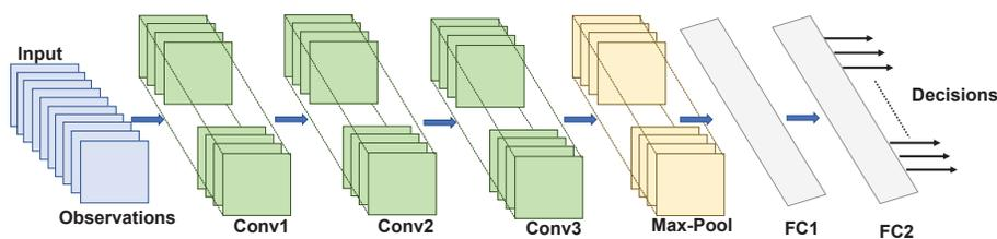
Fig. 3. Deep Q-Network Architecture
